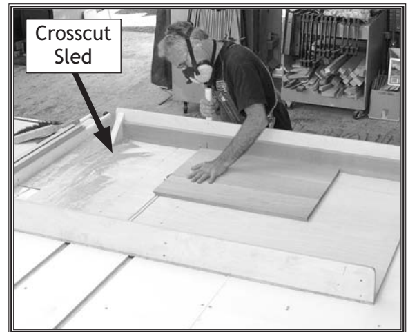
Figure 89. Example of crosscut sled.
